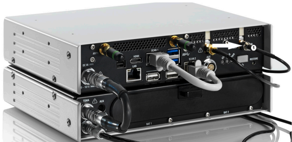
Figure 5-7: R&S TSMA Antenna Cabling - RF
