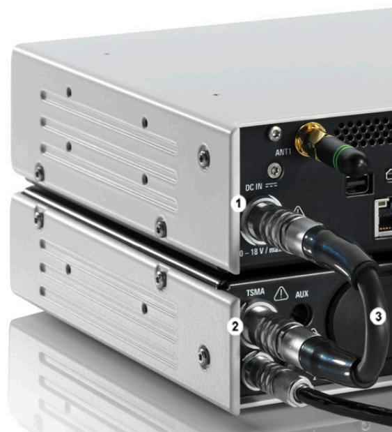
Figure 2-10: Cabling of R&S TSMA with R&S TSMA
