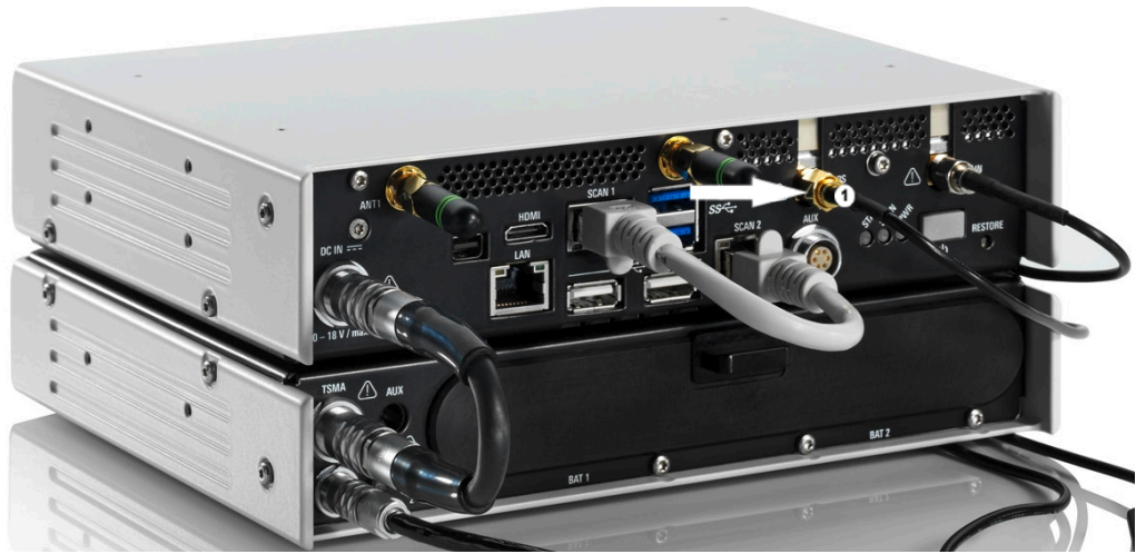
Figure 5-6: R&S TSMA Antenna Cabling - GPS
