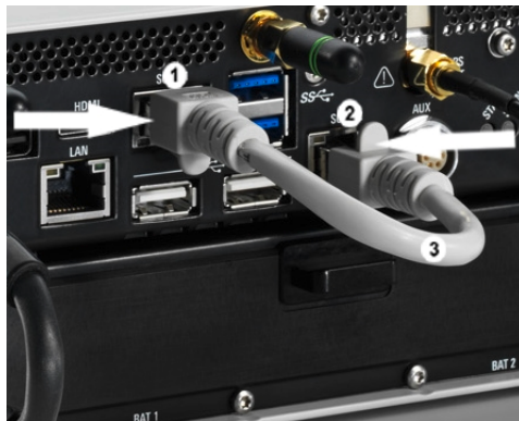
Figure 5-9: Connection between scanner unit and internal PC unit
