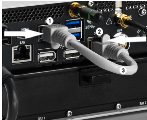
Figure 2-2: Connection between scanner unit and internal PC unit
