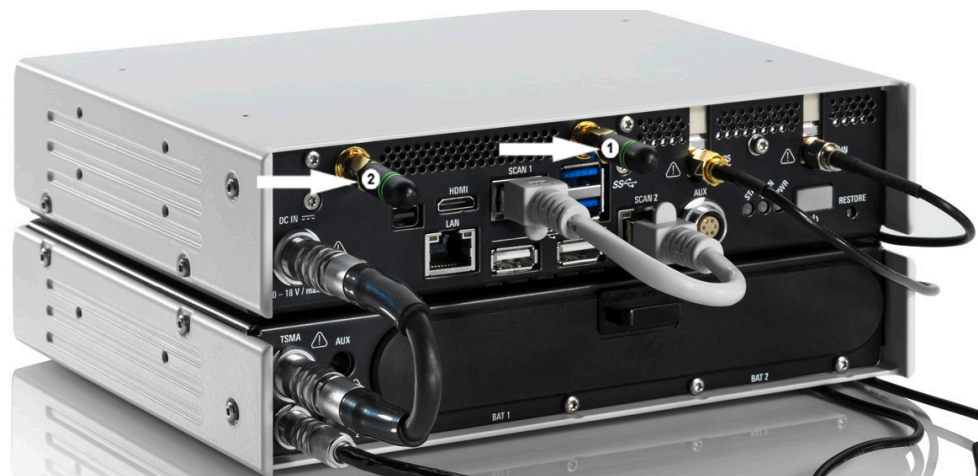
Figure 5-8: R&S TSMA Antenna Cabling - WLAN and Bluetooth
